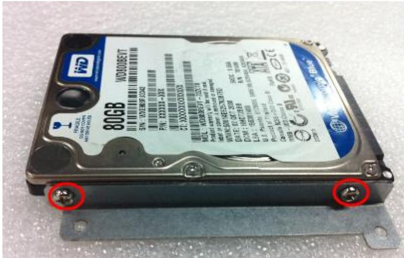
**Step 4** Fix the HDD bracket into the system, and plug the data and power cables to HDD. Installation completed.
