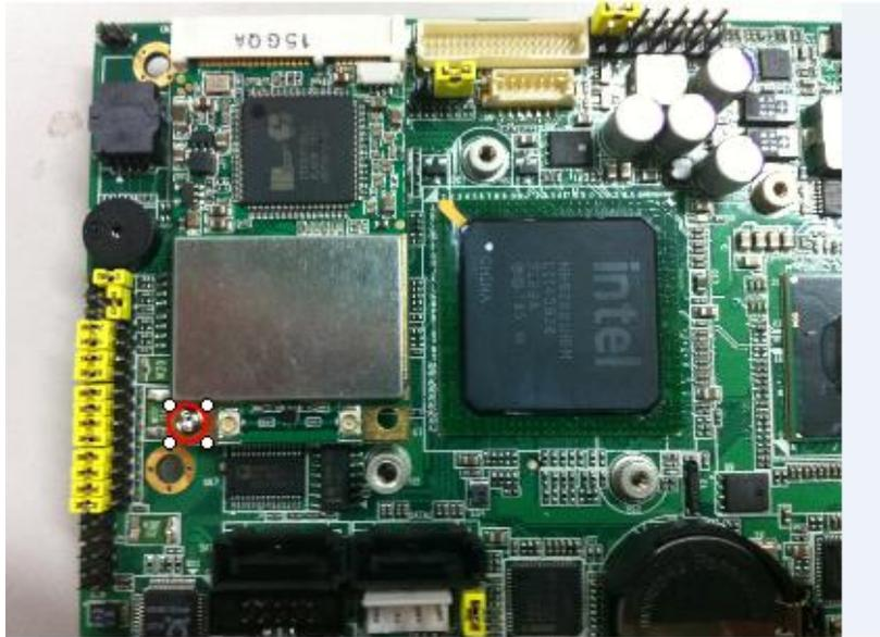
**Step 4** Connecting the Antenna cable with wireless LAN card
