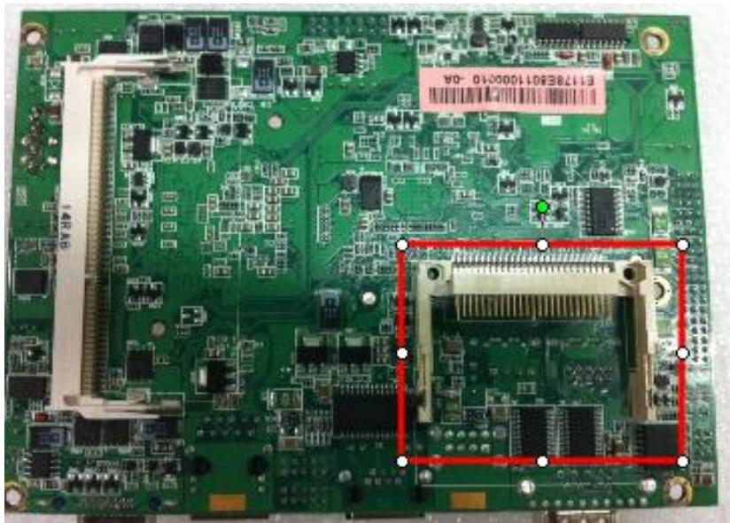
**Step 2** Insert the card into the socket, Installation completes.
