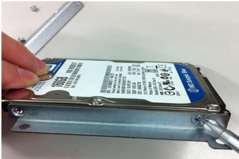
**Step 3** Fix the HDD on bracket by 4 screws at the side corner.
