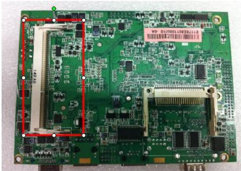
**Step 2** Pulg DDR3 667/800MHz SODIMM 204-pin memory into slot with angle of 45°
