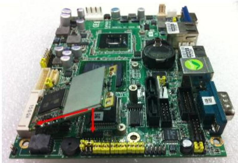
**Step 3** Fix the card on the M/B by a screw (M2x3L) at the side corner.
