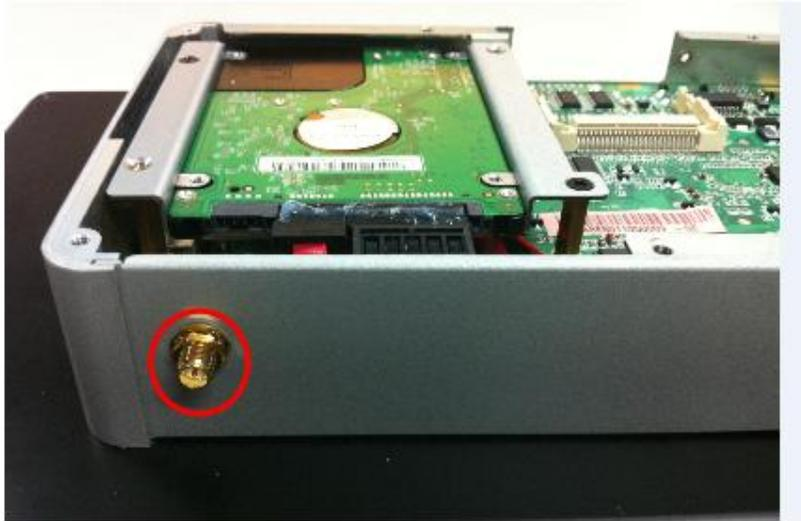
**Step 5** Install the antenna on the antenna connector.
