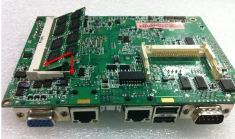
**Step 3** Press the memory into slot.
